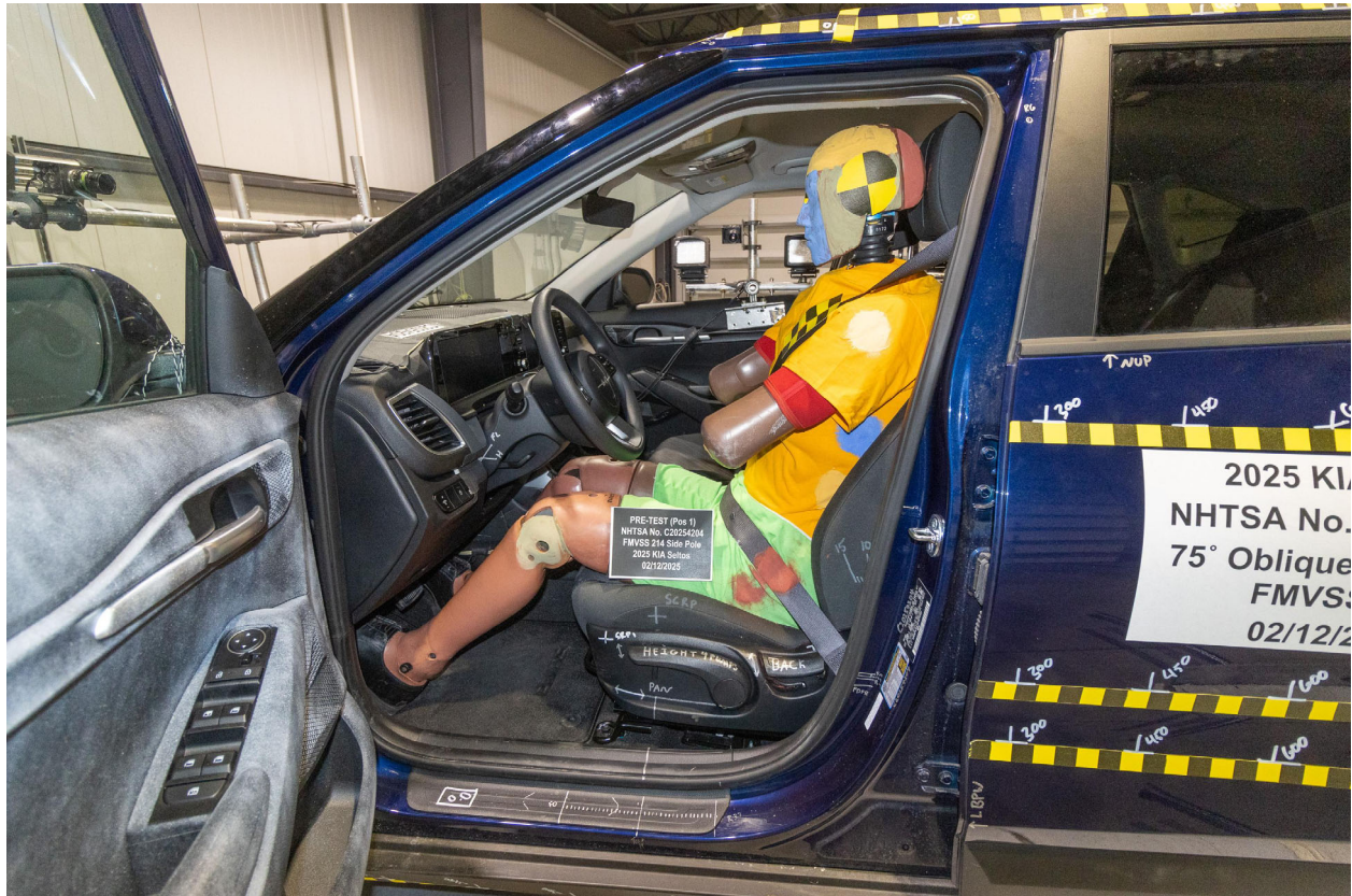
Figure A-15: Pre-Test Dummy with Door Open
